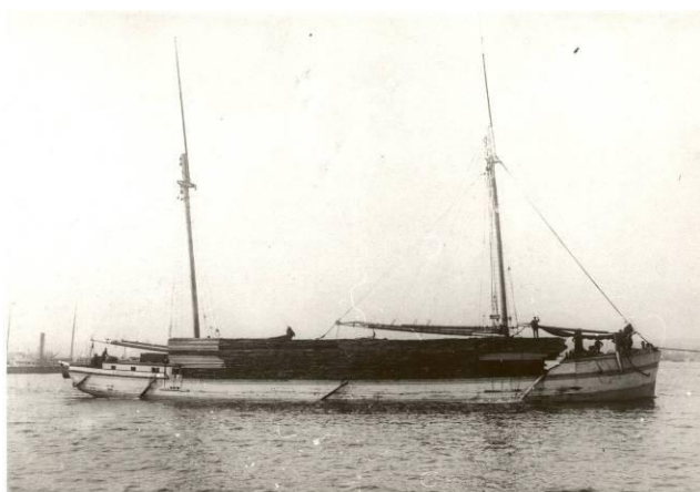
Figure 8. Originally built as a three-masted schooner, the 162-foot Harvey Bissell was later retrofitted to a two-masted "schooner barge," a typical conversion for schooners whose owners sought to keep the aging vessels in use. Pictured here with an enormous deck load of lumber, the Bissell wreck sits in 15 feet of water just off the Alpena waterfront. (Thunder Bay Sanctuary Research Collection)
